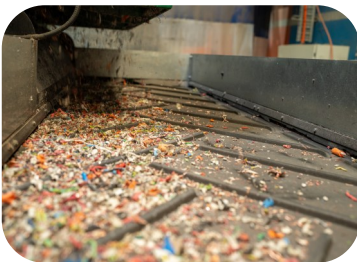
PVC/Vinyl is separated from the copper
